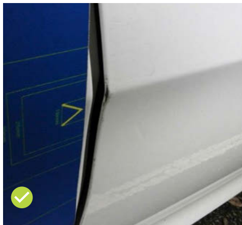
Small areas of chipping, including door edge chipping, are acceptable.
