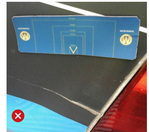
Scratches and abrasions over 25mm are not acceptable. Any scratch where the primer or base metal is shown will also be recharged.
