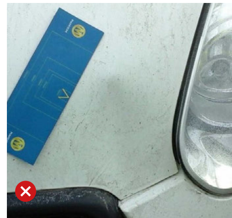
Dents over 15mm in diameter, or any dents to the roof or swage line on any panels, are not acceptable.
