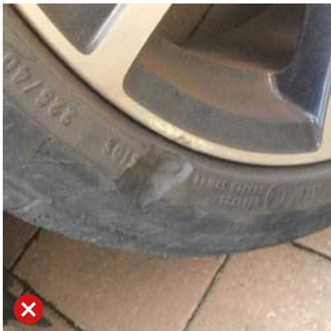
Tyre side wall damage is not acceptable.
