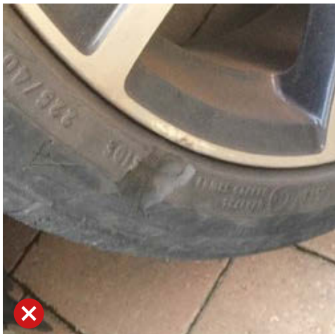
Tyre side wall damage is not acceptable.
