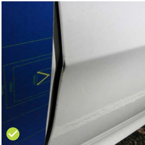
Small areas of chipping, including door edge chipping, are acceptable.
